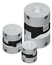
OLDHAM-FLEX couplings are based on the use of a disc that can move radially with respect to the two shafts, which permits the compensation of large misalignment errors between them.
